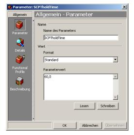
The selected parameter can be set by calling up the parameter properties window (selecting the "Properties" entry in the context menu). For more detailed information on the value range and the function, refer to the corresponding device documentation from the manufacturer.
