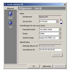
The neuron-ID of the new device is assigned to the database. The transfer of the neuron-ID can also be done here with the service pin or by entering it in the "neuron-ID" field.
