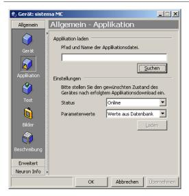
The application can be loaded for the individual device directly from the device properties window.
