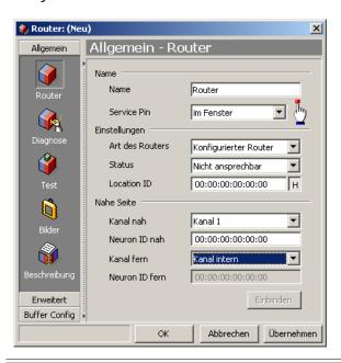
A name for the router is assigned and the type of router used is entered.
