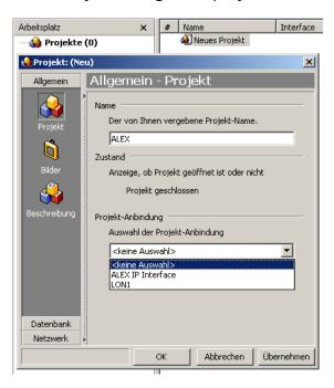
The name of the project is assigned here. The project connection (LON interface) can already be assigned.
