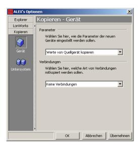
Parameters: The configuration of the source device can be taken over or a description of the parameters with the LON default values can be made.
