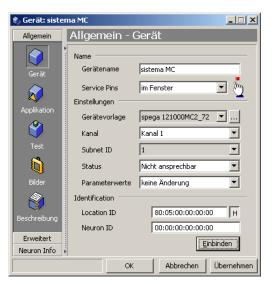
For picking, the devices must be assigned the respective neuron-ID. This can be done by entering it in the "neuron-ID" field or by pressing the service pin on the device.
