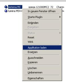
Loading can also be done for the individual device via the context menu. This opens the page of the properties window shown above.
