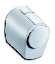
The actuator A24-10xx is a noiseless and maintenance-free continuous electrothermal actuator that is suitable for connection to clima RCM CC, clima RO-CC, clima AA4-10V, clima AA8-10V or clima FCB-10V. The control signal is a 0-10V analog signal.
